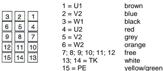
**Particularities:** The external rotor motor is equipped with thermal contacts which are embedded in the windings. These temperature-dependent circuit elements are monitoring the winding temperature of the motor. If properly connected, the fan is thus protected from overload, mains phase failure, lock-breaking of the motor and too high ambient operating temperatures. Maintenance-free operation is ensured by means of ball-bearings with long-term lubrication which are closed on both sides.
